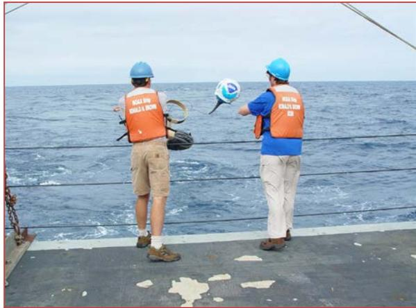
*The modern drifter is a high-tech version of the "message in a bottle". Drifting buoys measure sea surface temperature and are used to track ocean currents. The drifter's data are transmitted to a satellite and received in near real-time at the Adopt a Drifter Program website ([www.adp.noaa.gov](http://www.adp.noaa.gov)).*
