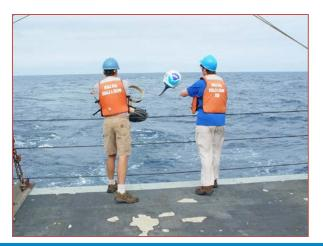
The modern drifter is a high-tech version of the "message in a bottle". Drifting buoys measure sea surface temperature and are used to track ocean currents. The drifter's data are transmitted to a satellite and received in near real-time at the Adopt a Drifter Program website (www.adp.noaa.gov).
